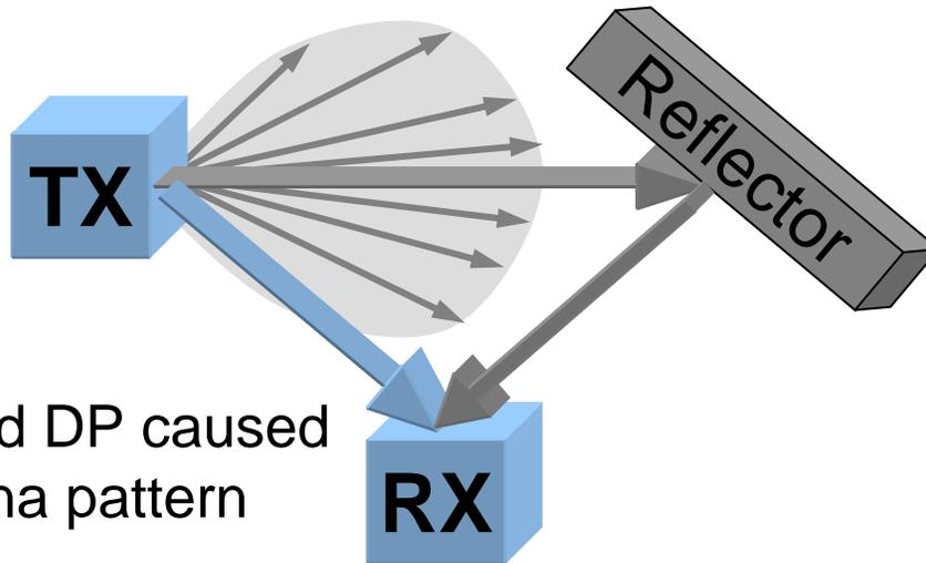
An attenuated DP caused by the antenna pattern
