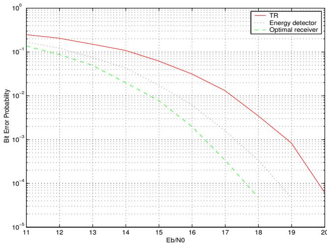
Figure 3: BER of the standard TR-UWB ("TR"), the two-point constellation proposed here with an energy detector ("Energy Detector"), and the two-point constellation proposed here with an optimal receiver based on Section 3 ("Optimal Receiver") for a fixed multipath channel, versus the signal-to-noise ratio  $\frac{E_b}{N_0}$ , where  $E_b$  is the total received energy per information bit.
