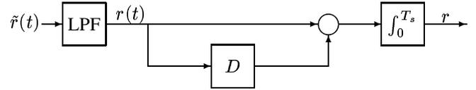
Figure 1: Receiver for a standard TR-UWB communication system, where  $\hat{r}(t)$  is the received signal, and  $r(t)$  is a lowpass-filtered version of such. The signal is multiplied by a delayed version of itself and the result integrated over the symbol period  $T_s$ , which can consist of many frames, each of duration  $T_f$ , in low data rate UWB systems. A threshold decision is made on  $r$  to decode the data bit for the current symbol.
