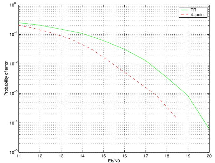
Figure 5: Bit error probability of the four-point constellation described in the text with an optimal receiver based on Section 3 ("4-point") and of standard transmitted-reference ("TR") for a fixed multipath channel, versus the signal-to-noise ratio  $\frac{E_b}{N_0}$ . Note that the proposed four-point system is transmitting data at twice the rate of the transmitted-reference scheme, while preserving the same timing requirement and with performance as shown.
