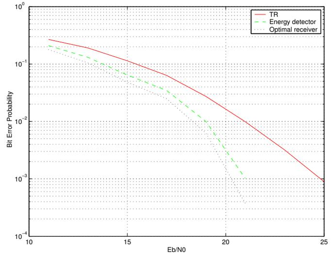
Figure 4: Bit error probability of the standard transmitted-reference ("TR"), the two-point constellation proposed here with an energy detector ("Energy Detector"), and the two-point constellation proposed here with an optimal receiver based on Section 3 ("Optimal Receiver"), averaged over the multipath fading, versus the signal-to-noise ratio  $\frac{E_b}{N_0}$ , where  $E_b$  is the average total received energy per information bit.
