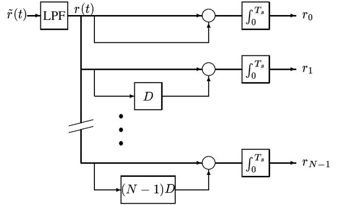
Figure 2: Receiver front-end for the proposed generalized transmitted-reference system. Note that, instead of a threshold rule being applied to each of the outputs  $r_i$ , a joint decision is made on  $\underline{r}$  to decode each symbol, as described in the text.
