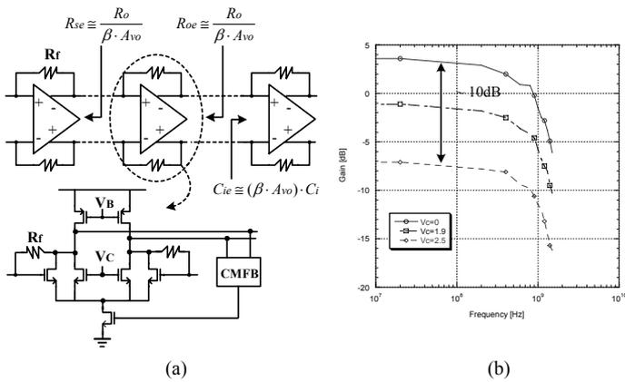
Figure 18.5.3: (a) 4-stage feedback LPF. (b) Gain response.
