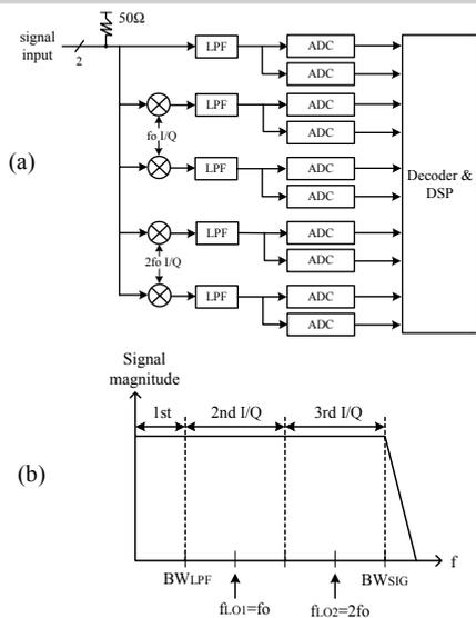
Figure 18.5.1: (a) Receiver architecture. (b) Frequency relationship.
