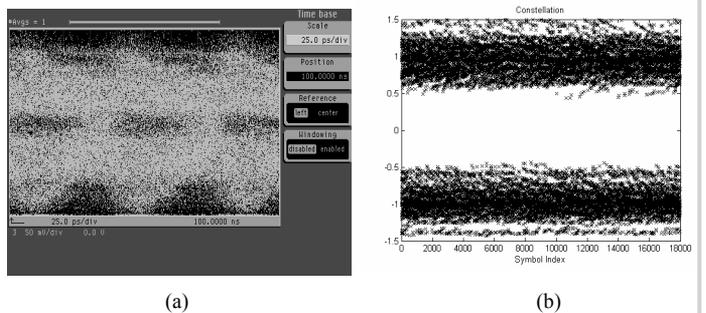
Figure 18.5.6: (a) Eye diagram at receiver input. (b) Slicer input after equalization.
