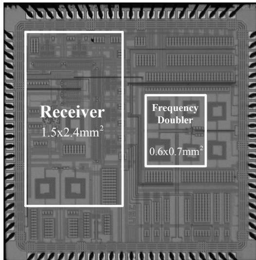
Figure 18.5.5: Chip micrograph.
