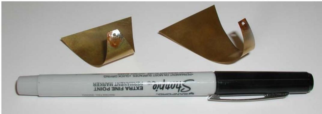
**Figure 7.** A few samples of the tongue flare used in prototype in Figure 6. The elements are soldered to the central pin of the coaxial SMA connector.
