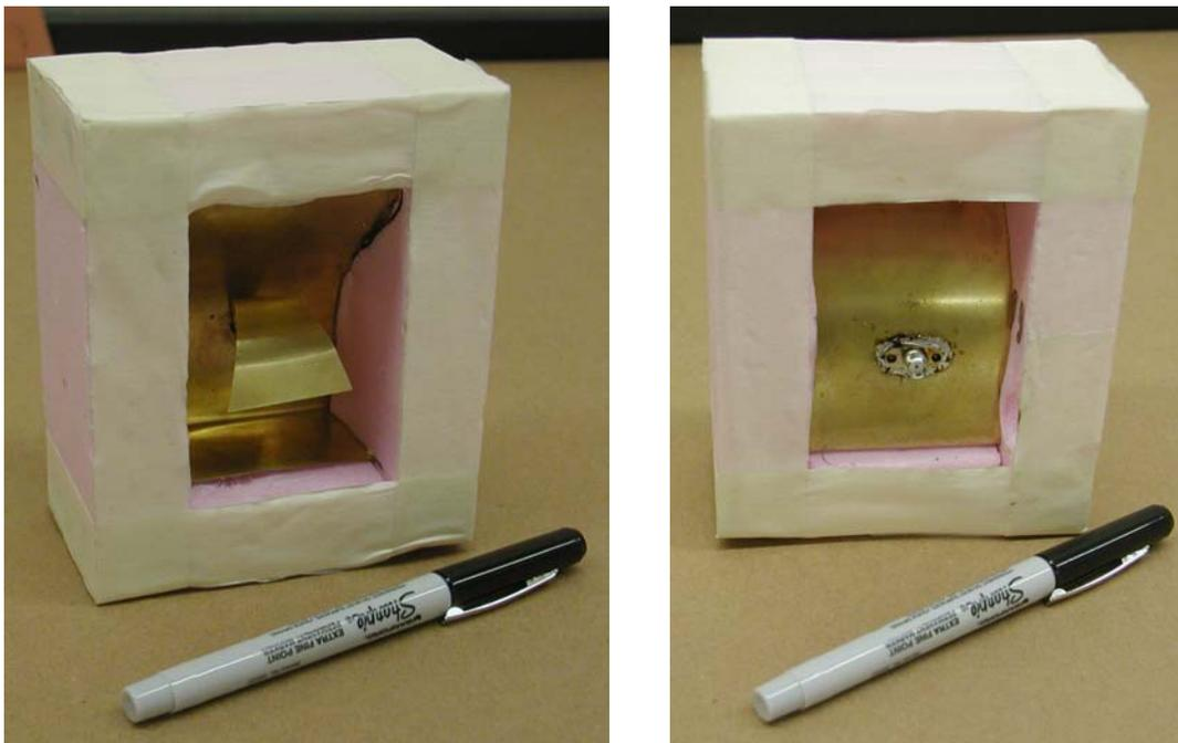
**Figure 6.** A compact prototype of UWB antenna operating in the 2-10 GHz band: (a) front view; (b) backside view with SMA coaxial connector. A foam support surrounds the antenna. In production, the reflector can be fabricated from self-supporting material, eliminating the need for external support.
