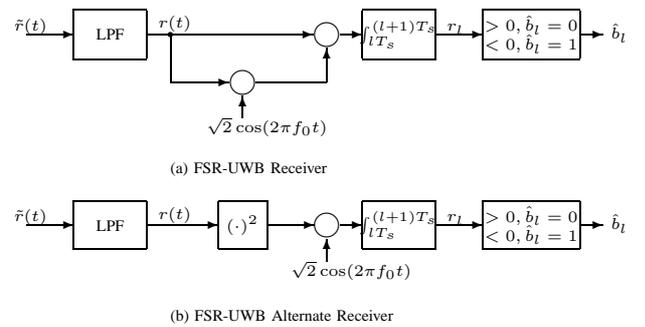
Fig. 2. (U) Receiver for the proposed FSR-UWB system. Note that the delay element in Figure 1 has been replaced by a mixer in (a). Since multiplication is commutative, the receiver in (a) can be drawn in the more convenient form given in (b).
