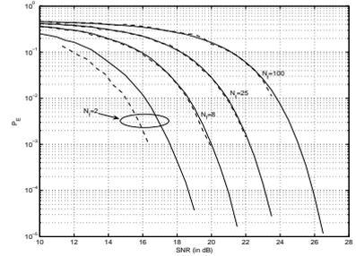
Fig. 3. (U) The bit error probability versus average signal-to-noise ratio for the proposed FSR-UWB system on an AWGN channel. Dashed lines correspond to simulation results, whereas solid lines correspond to the analytical results of (6).
