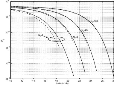
Fig. 4. (U) The bit error probability versus average signal-to-noise ratio for the standard TR-UWB system on an AWGN channel. Dashed lines correspond to simulation results, whereas solid lines correspond to the analytical results of (7).
