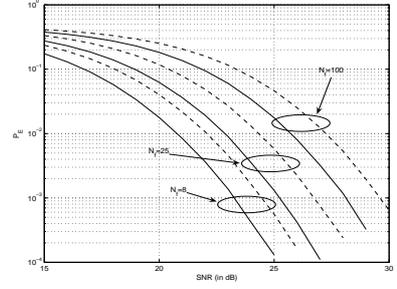
Fig. 5. (U) The bit error probability versus average signal-to-noise ratio for the TR-UWB system (dashed lines) and FSR-UWB system (solid lines) operating over a multipath fading channel. The system parameters are the same as those for Figure 3. Results are obtained by generating  $10^5$  random channels  $\underline{h}$  for each data point and using such to empirically estimate the expectations in (9) and (10).
