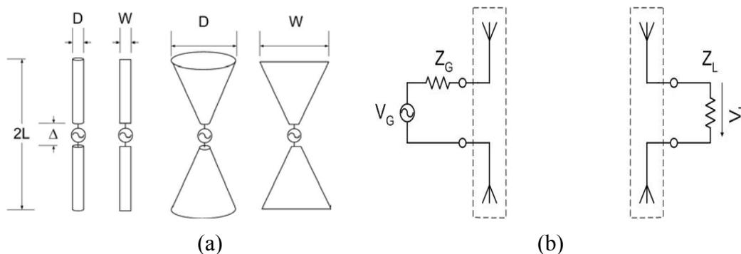
**Fig. 1.** (a) Geometrical templates for several practical dipoles including 3-D solid and 2-D flat structures with parameterized length  $L$ , diameter  $D$  and width  $W$ . (b) Two-antenna link model with transmitter generator and receiver load connected to antenna ports.
