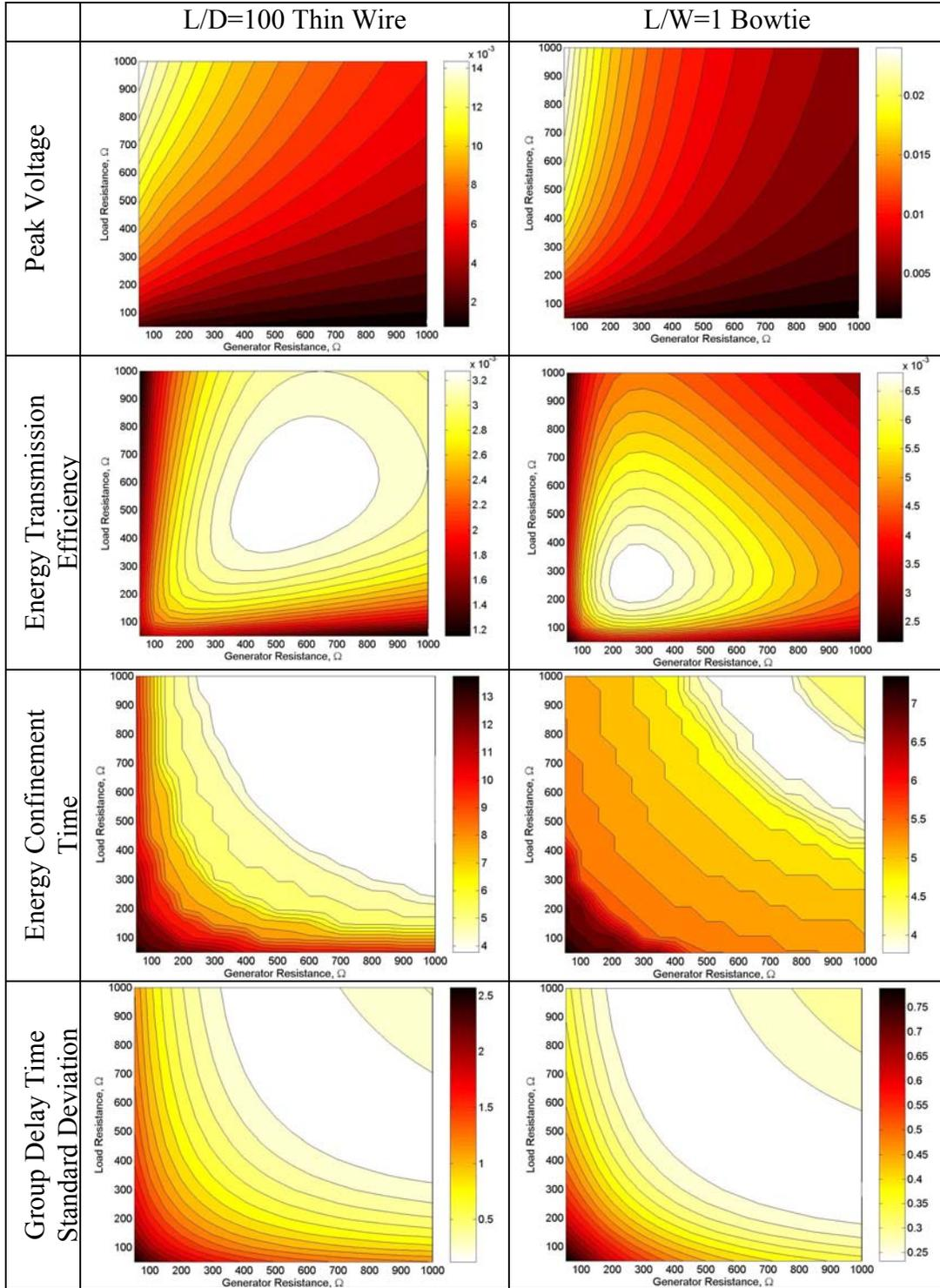
**Fig. 2.** Link performance measures versus the resistive loads for thin wire ( $L/D=100$ ), at the left, and flat bowtie ( $L/W=1$ ), at the right. Peak voltages are multiplied by  $R$  from (2). Energy transmission efficiencies are multiplied by  $R^2$  from (2). Time units are multiplied by  $1/\tau_0$ , where  $\tau_0 = L/c$  is traveling time along the dipole arm, Fig. 1a.
