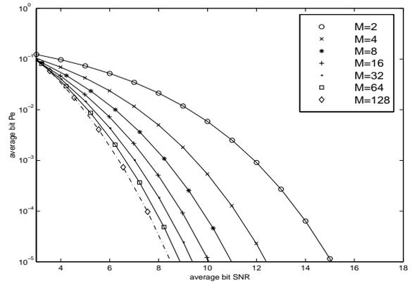
Fig. 2. The  $\overline{\text{UBPb}}\left(\frac{\overline{E}_{\Psi}}{N_o}\right)$  Curves for  $M = 2, 4, 8, 16, 32, 64$  signals.
