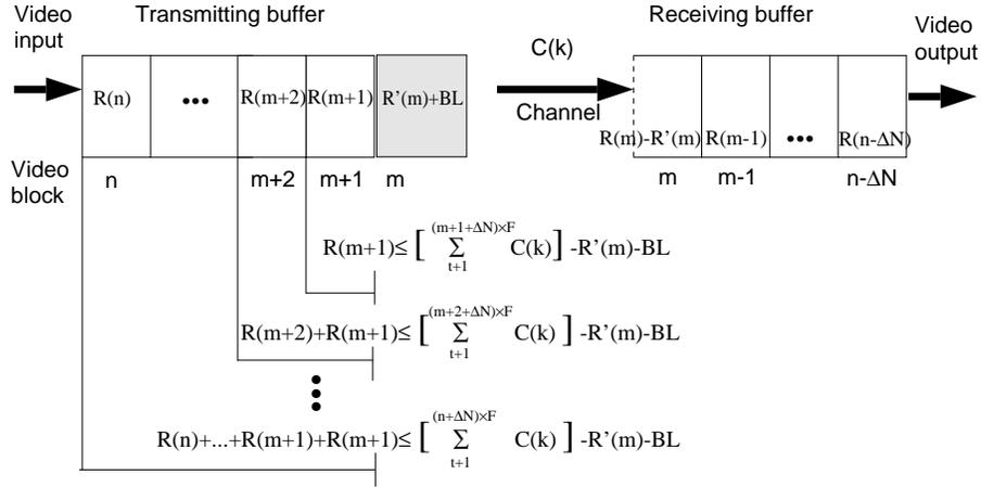
Fig. 2. Constraint on encoding rate for each buffered video block at time  $t$ .
