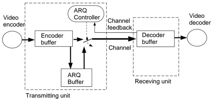
Fig. 4. Diagram of buffers in the system
