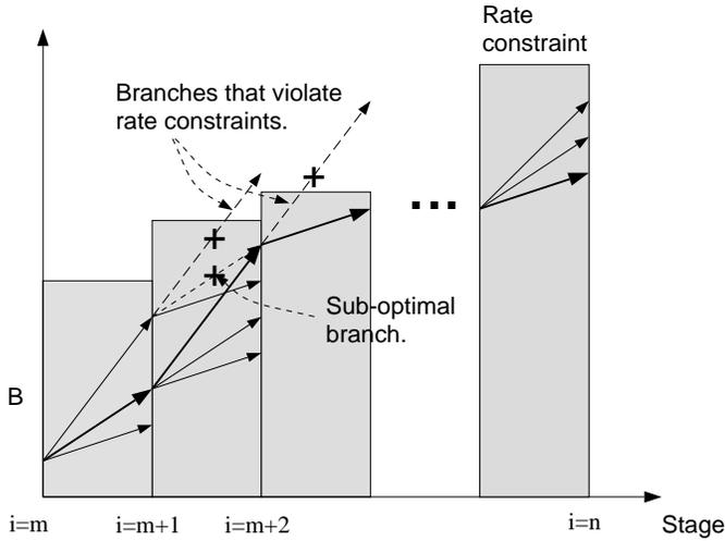
Fig. 7. Trellis tree in dynamic programming for searching the optimal encoding rate allocation.
