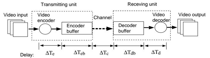
Fig. 1. Delay components of a communication system.
