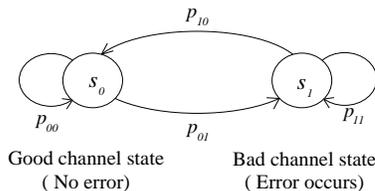
Fig. 5. Two state Markov channel model.
