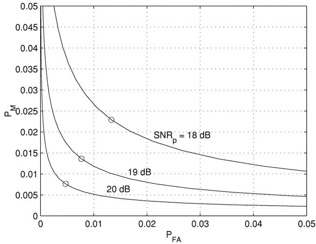
Fig. 5. Early false alarm probability versus probability of a missed direct path for different peak SNRs.  $\theta_\delta = 100$  ns and  $\theta_\rho$  was varied. At the circular mark on each curve, probability of error is minimized.
