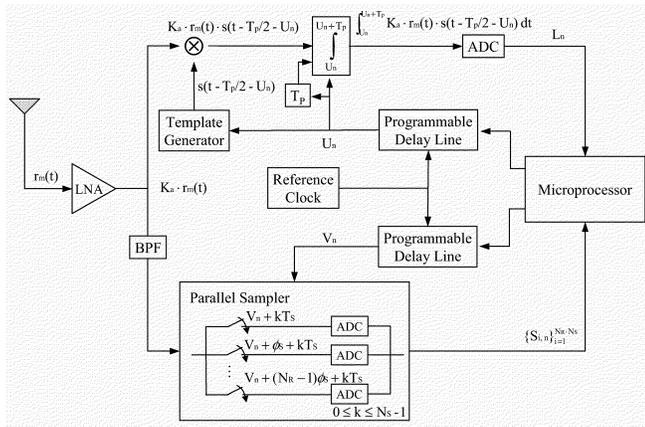
Fig. 8. Receiver schematic of UWB ranging system.
