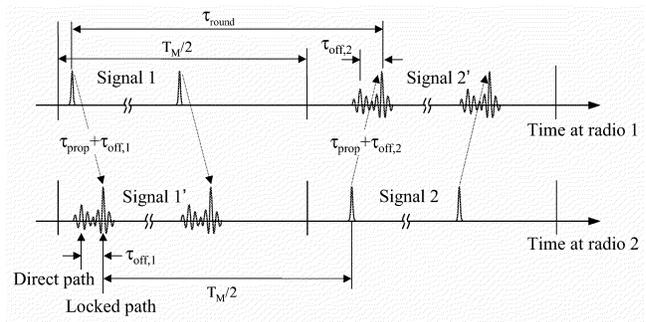
Fig. 9. Evaluation of the signal round-trip time.
